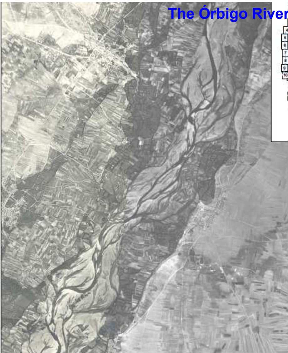
Comparison between orthophotos of a 5 km segment in the Stretch I of the Órbigo River taken in 1956 and 2006. They show perfectly the encroachment on the original channels (braided), the channelization and the drastic morphological changes occurred in 50 years.
